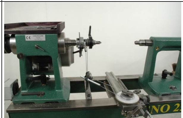
Ø 35 mm dividing head on spindle Ø 55 mm on spool on the lower linear bearing
