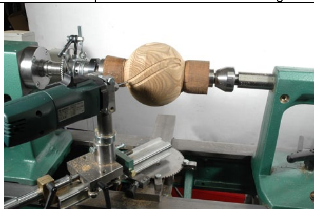
Ø 45 mm dividing head on spindle Ø 30 mm on spool on the lower linear bearing
