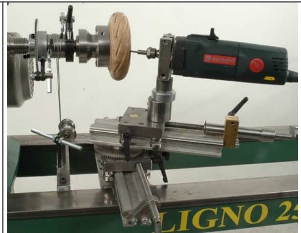
Ø 45 mm dividing head on spindle Ø 30 mm on spool on the lower linear bearing
