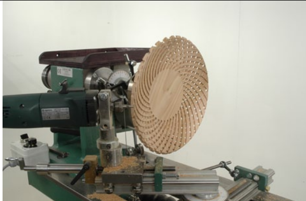
Ø 35 mm dividing head on spindle Ø 55 mm on spool on the lower linear bearing
