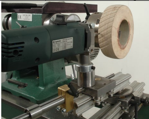
Ø 35 mm dividing head on spindle Ø 30 mm on spool on the lower linear bearing
