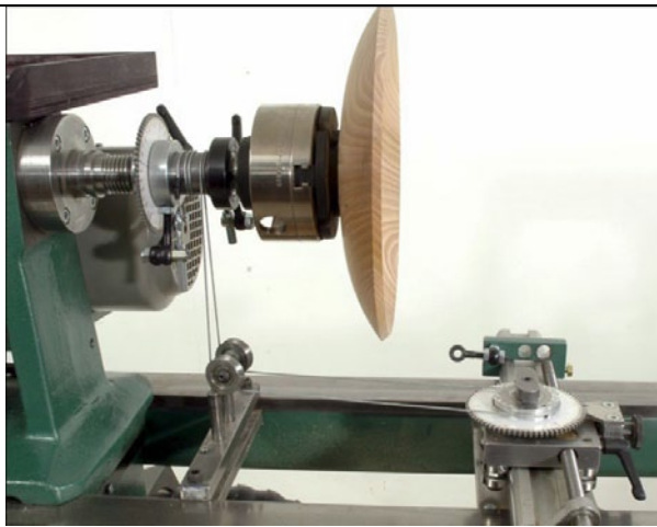
Ø 35 mm dividing head on spindle Ø 55 mm on spool on the lower linear bearing
