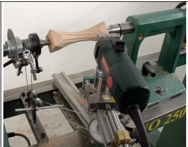
Ø 35 mm dividing head on spindle Ø 55 mm on spool on the lower linear bearing
