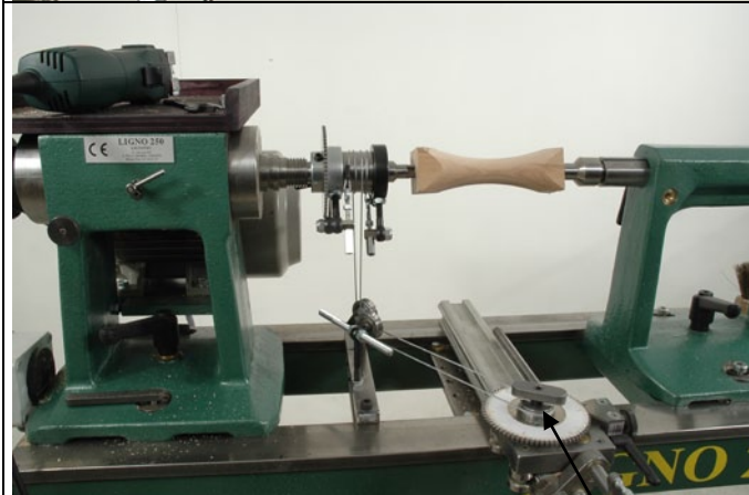
The wire is mounted on the smallest diameter spool.
