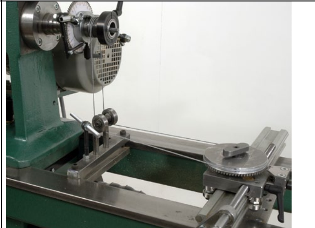
The wire is mounted on the biggest diameter spool.
